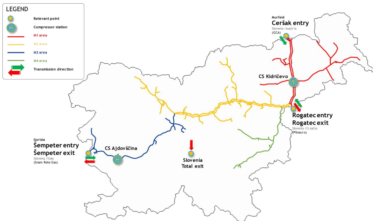
Figure 4. Schematic map of the gas transmission system with relevant points
